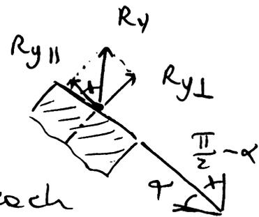
Just pay attention to the sign of each contribution, considering that  $N$  is negative in the case of compression force,  $V$  is positive if related to an ideal clockwise rotation of a small element of structure,  $M$  is positive when "inferior fibres" are under tension  $\rightarrow$  for the sake of simplicity, when FRP is applied  $M$  tends to put in tension the side where FRP is applied
