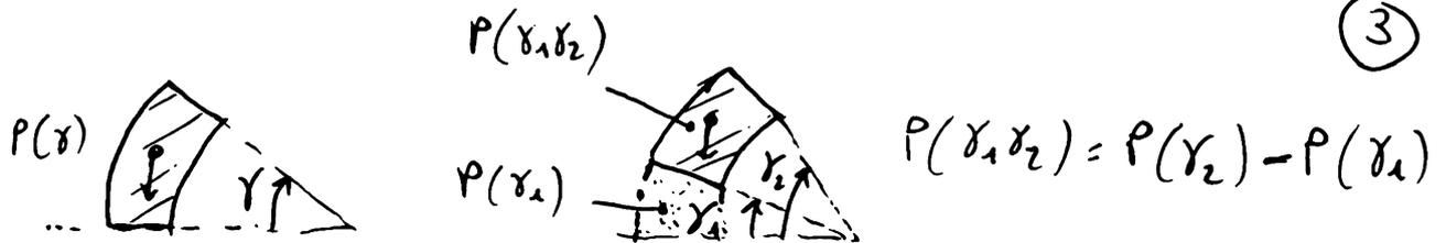
$$W = b \cdot (P(\gamma_c) - P(\gamma_A)) = b \cdot R \cdot \frac{\gamma_c - \gamma_A}{2} (R_c^2 - R_i^2)$$
