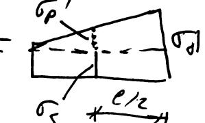
$$\text{quindi } \sigma_p = \sigma_s + \sigma_p' = \sigma_s + \frac{1}{2} \sigma_d - \frac{1}{2} \sigma_s = \frac{1}{2} (\sigma_s + \sigma_d) = \sigma_0$$
